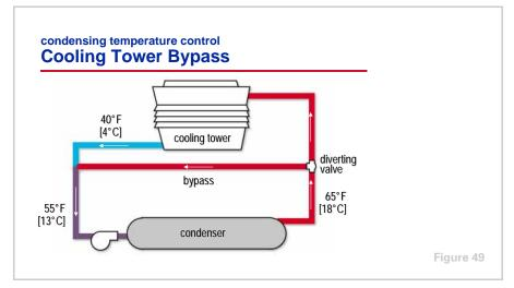
Controlling the refrigerant pressure difference between the evaporator and condenser of a water-cooled chiller is accomplished by varying the temperature or flow rate of the water flowing through the condenser. The following are 5 common methods used to control condensing temperature:
